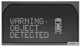
The vehicle is close to the obstacle when the EVIC display shows one flashing arc and sounds a continuous tone. The following chart shows the warning alert operation when the system is detecting an obstacle:
